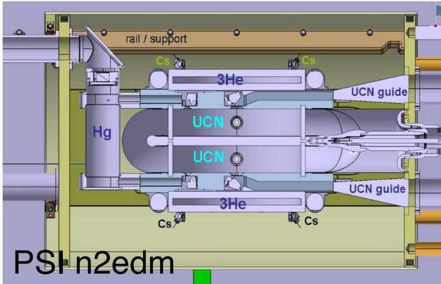
both have 2 UCN chambers, Hg comag, additional outer magnetometry cells, additional external Cs magnetometers
