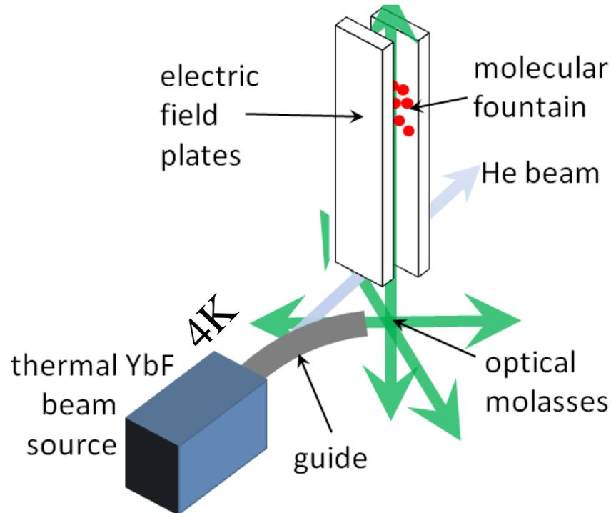
*Design for a fountain of YbF molecules to measure the electron's electric dipole moment*
