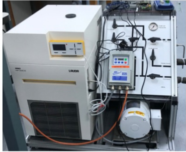
Chiller/pump co-designed with RAL
