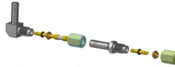
Design of demountable high pressure cooling couplings, facilitating stave testing and giving significant cost savings compared to baseline.
