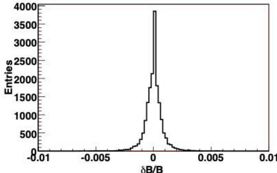
**Figure 4.2:** Relative difference between the measurements of  $B$  using different Hall probes at the same position in the magnet. The resolution is completely dominated by the precision of the calibration of the Hall probes.
