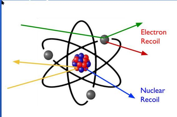
Electrons and gammas interact with atomic electrons, producing electron recoils (ER).
