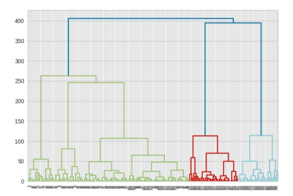
We can use this to approximate number of clusters needed by drawing a line across where the bigger sub-clusters are and seeing how many lines we intersect. Another method is the elbow plot which uses k-means itself to find where the error rate begins to smooth out. An example where the correct number of clusters is five is shown below.
