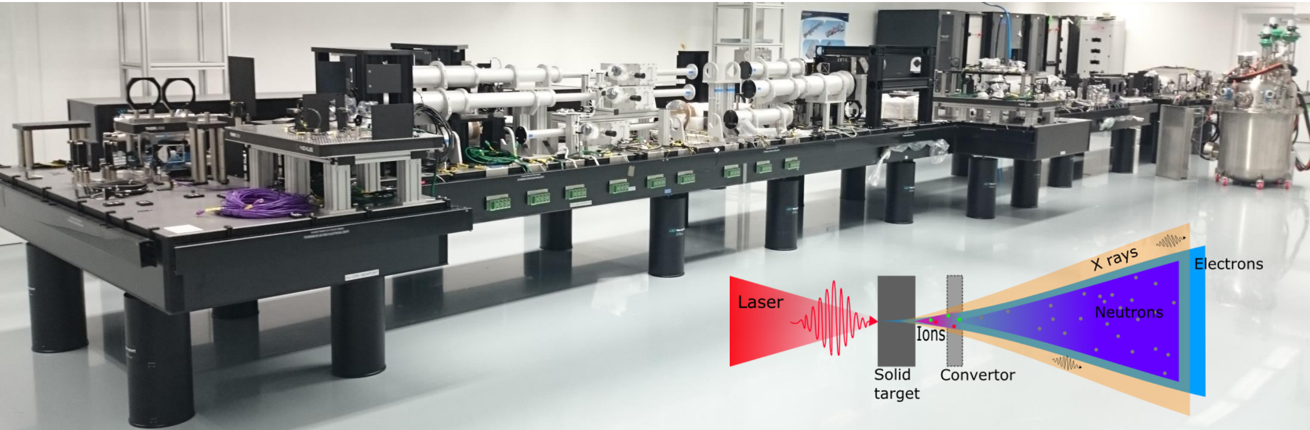
CLF's world leading 10 Hz 100 J laser DiPOLE100
