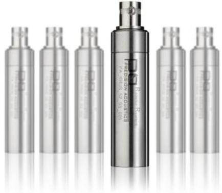
Designed for ambient temperature inspection and NDT applications in high radiation environments, Precision Acoustics' Radiation resilient RRUS transducers have been tested up to a cumulative Gamma dose of 9.5 MGy with almost no change in performance up to doses of 2 MGy.
