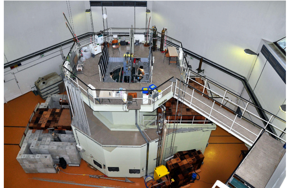
Nuclear reactor for neutron and gammas damage studies.
